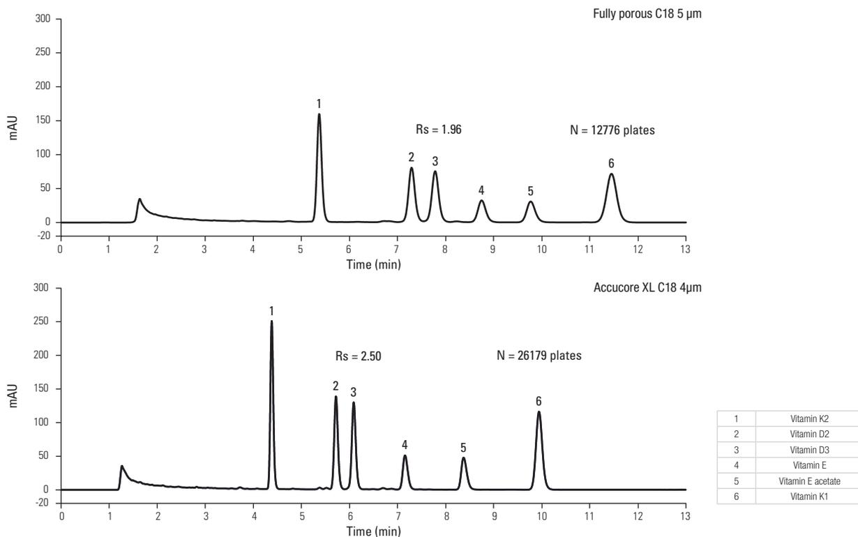
Figure 1: Comparison of the resolution of a critical pair (peaks 2 and 3) on 5  $\mu\text{m}$  fully porous C18 and 4  $\mu\text{m}$  Accucore XL C18 HPLC columns. Experimental conditions: columns – 150 x 4.6 mm; mobile phase – acetonitrile / methanol (80:20 v/v); flow rate – 1 mL/min; column temperature – 30  $^{\circ}\text{C}$ ; UV detection – 280 nm; injection volume – 5  $\mu\text{L}$ .
