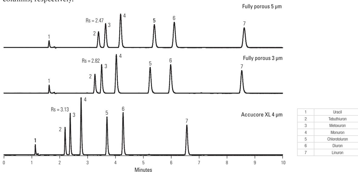
Figure 2: Comparison of the resolution of a critical pair (peaks 2 and 3) on fully porous 5 and 3  $\mu\text{m}$  and Accucore XL 4  $\mu\text{m}$  HPLC columns. Experimental conditions: columns – C18, 150 x 4.6 mm; mobile phase – water and acetonitrile; gradient – 35% to 60% acetonitrile in 10 min; flow rate – 1 mL/min; column temperature – 30  $^{\circ}\text{C}$ ; UV detection - 247 nm; injection volume – 5  $\mu\text{L}$
