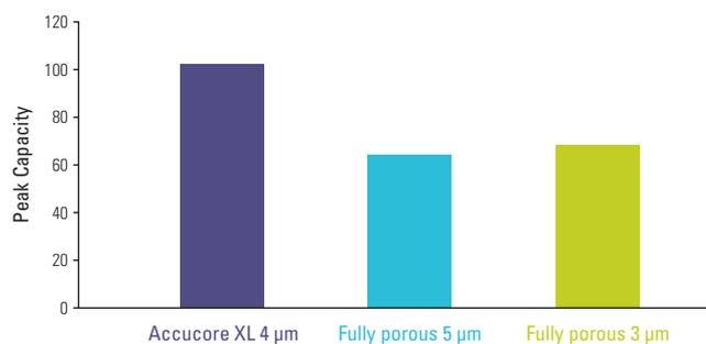
Figure 3: Peak capacity comparison for the herbicides method
