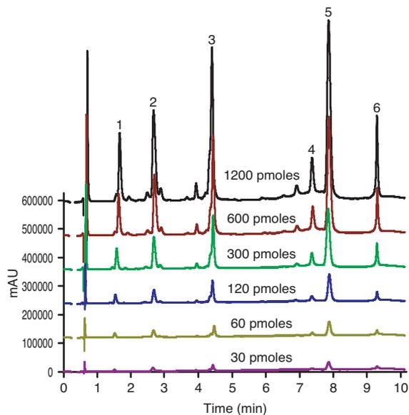
Figure 2: UV chromatograms showing the result of different loads of six protein mix. The total protein picomolar load on the column is reported
