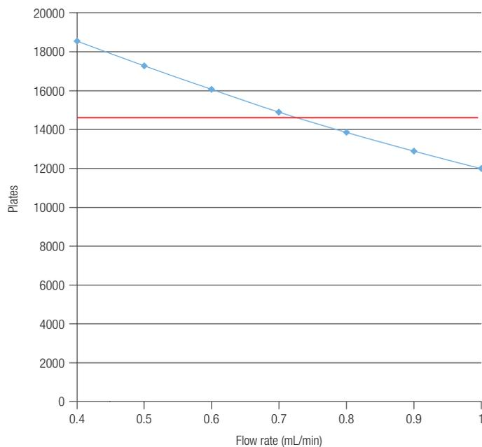
**Figure 4. Plate count values when increasing the method flow rate on an Accucore C8, 100 × 2.1 mm, 2.6 μm column. The red line represents the 80% value of the plate count at 0.4 mL/min and the limit for USP equivalence.**
