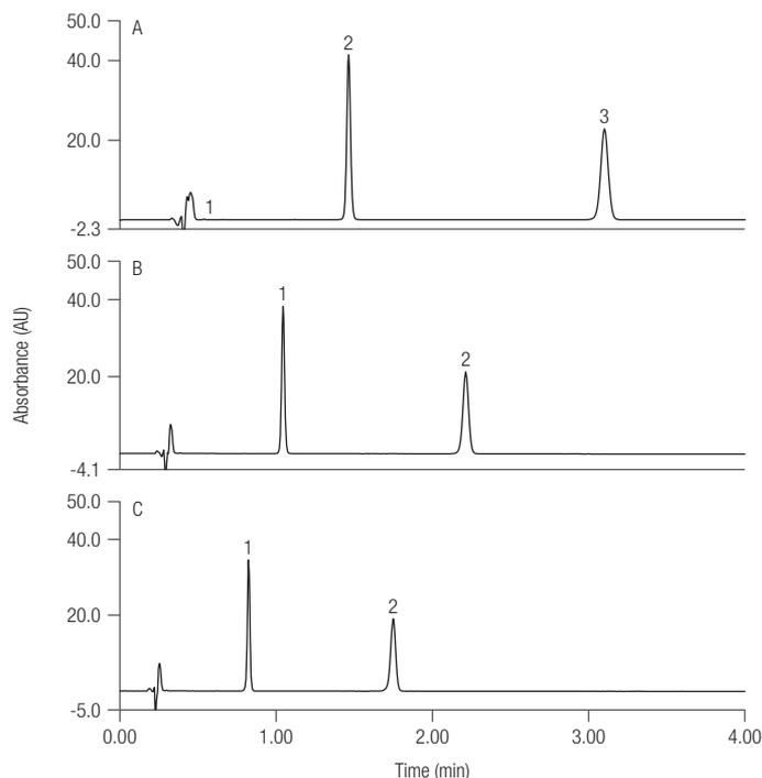
**Figure 3. Representative chromatograms observed when increasing the method flow rate on an Accucore C8, 100 × 2.1 mm, 2.6 μm column.**
