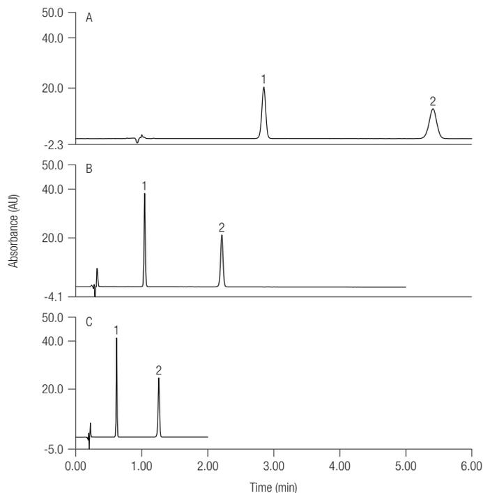
**Figure 7. A comparison of the key stages of the method development. A) Original USP method, Hypersil GOLD, 150 mm × 4.6 mm, 5 μm column, 2 mL/min, 25 °C, B) Scaled USP method, Accucore C8, 100 × 2.1 mm, 2.6 μm column, 0.7 mL/min, 25 °C, C) Beyond USP method, Accucore C8, 100 × 2.1 mm, 2.6 μm column, 1.0 mL/min, 45 °C**
