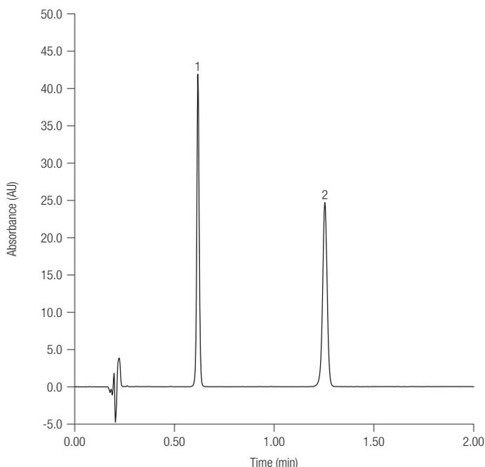
**Figure 8. Overlay of 24 replicate injections of the standards mixture using the final developed method on an Accucore C8, 100 × 2.1 mm, 2.6 μm column, 1.0 mL/min, 45 °C.**
