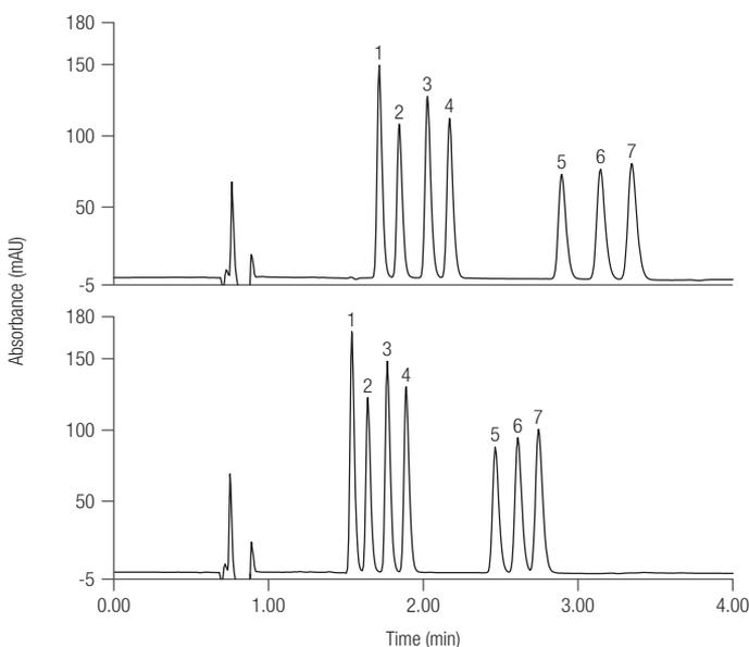
**Figure 2. Chromatogram showing mixed standards analyzed at two different column temperatures a) 50  $^{\circ}\text{C}$  and b) 60  $^{\circ}\text{C}$ .** (1) prednisone, (2) cortisone, (3) prednisolone, (4) hydrocortisone, (5) corticosterone, (6) betamethasone and (7) dexamethasone.
