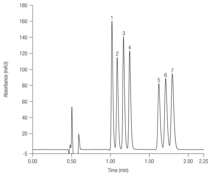
**Figure 5. Overlay of 24 replicate injections of standards mixture at 60 °C and a flow rate of 0.6 mL/min.**
